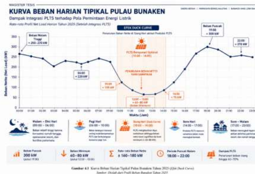
Figure 2. Typical daily load curve for Bunaken Island Source: PT PLN (Persero) load data, processed by the authors, 2024
